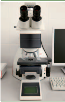
Fluorescent microscope DM4000 – fully automated microscope with motorized parts for cytogenetic analysis, also suitable for FISH, mFISH, and CGH analyses. Device for evaluation of karyotypes and FISH analysis with digital camera is a part of the instrument.
