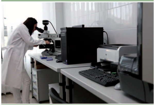
Fluorescent microscope DM4000 – fully automated microscope with motorized parts for cytogenetic analysis, also suitable for FISH, mFISH, and CGH analyses. Device for evaluation of karyotypes and FISH analysis with digital camera is a part of the instrument.
